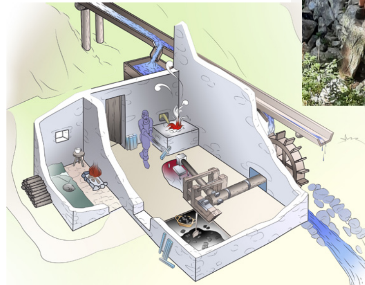
Hypothetical restitution of work at the Madriu ironworks (drawing, O. Vingolte)
